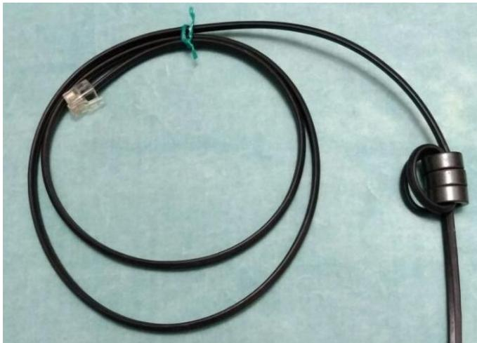
*Fig.9 Control cable with common mode balun*
