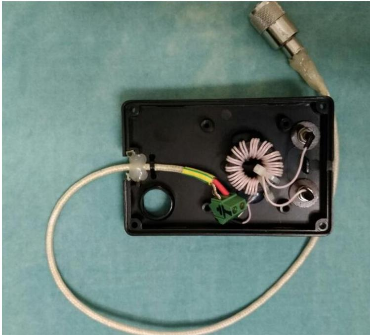
**Fig.10** Balun at the feeder output
