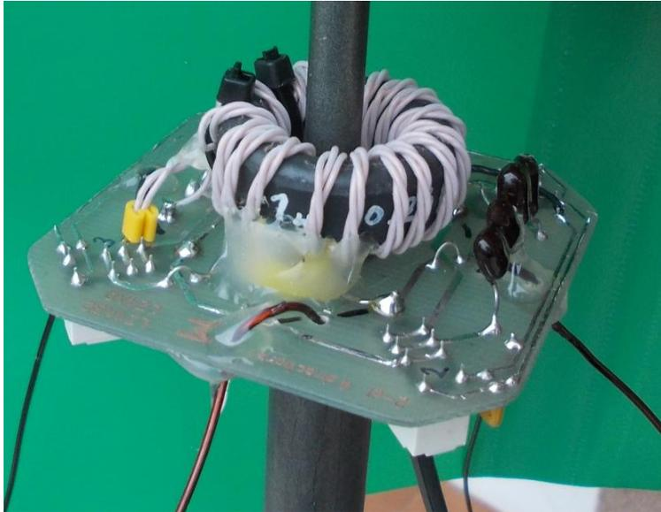
**Fig.8a** The transformer. The board is inserted into the top of the mast.
